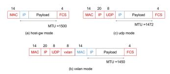
Figure 9: frame diagram
