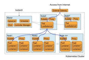
Figure 2: Kubernetes cluster with proposed load balancer.
